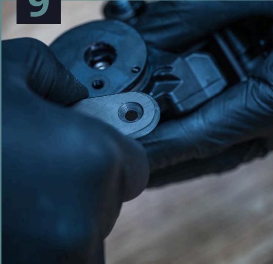
Align the OSPW system cage plate with the back of the derailleur, inserting the spring post into the low (L) tension setting on the cage (B). There's no need to worry about aligning the D-shaped interface at this stage.
