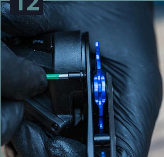
**Turn the OSPW system cage forward and insert the rotation stop screw with a 2.5mm hex key. Tighten it to a torque of 3.0Nm.**
