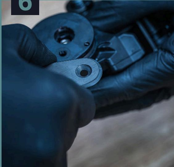
Using the **CyclingCeramic** front cage plate, turn the D-shaped center post inside the derailleur counterclockwise until it reaches the stop. Then, remove the cage plate.
