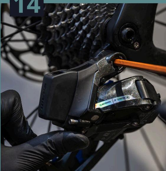
**Mount the derailleur onto the bike. Shift to the smallest cog (bottom gear) and then install the rear wheel.**
