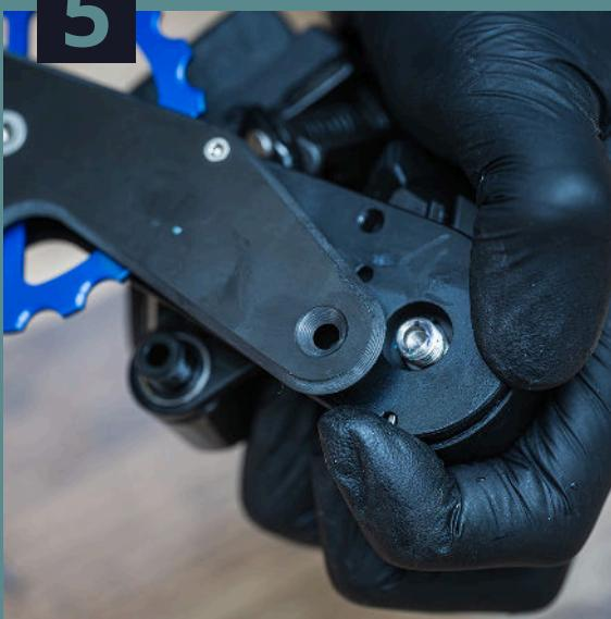
**Disassemble the OSPW system by removing all 4 bolts from the back of the system. Set aside the 4 bolts, back cage plate, and both pulley wheels.**
