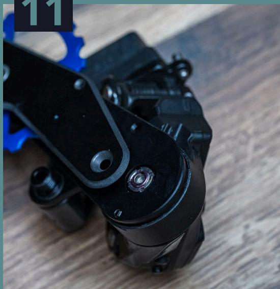
Once aligned, press the cage against the derailleur body to secure the D-interface. You should feel the cage lock into place. A slight wiggle may be needed to fully engage it. Then, using the included 4-pronged tool, tighten the center nut to a torque of 6Nm.
