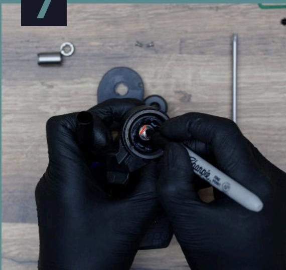
Use a marker to mark the end of the center screw, identifying the flat surface of the D-shaped interface at the bottom of the screw (A).
