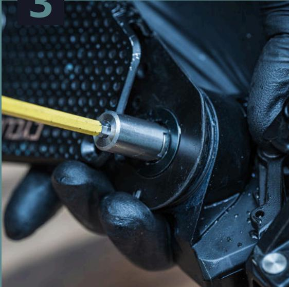
**Hold the stock pulley cage (not just the derailleur) and use the CyclingCeramic special tool to loosen the main center nut, but do not remove it completely. Once the center nut is sufficiently loose, allow the rotation stop screw to pass the stop point on the derailleur body, which will release the spring tension.**
