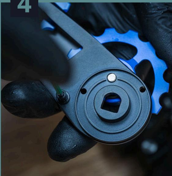
**Unbox the CyclingCeramic OSPW system and remove the rotation stop screw (to be reinstalled once the cage is mounted).**
