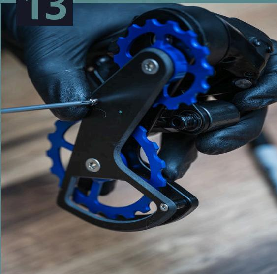
**Place the 14-tooth pulley on the upper post and the 19-tooth pulley on the lower post of the OSPW system cage, ensuring that all four spacers are correctly positioned and the pulleys are installed with the etching facing outward (towards the front cage plate). Align the back cage plate and fasten it by tightening the four 2.0mm cage bolts to a torque of 1.5Nm.**
