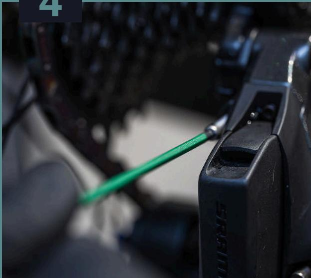
With the chain now cut to the correct length, it's crucial to check the clearance of the OSPW system when the rear derailleur is in the largest cog on the cassette. As indicated by the arrow, the cage should be able to rotate counterclockwise. Ensure there is adequate clearance between the upper pulley wheel of the OSPW system and the largest cog on the cassette. If the clearance is insufficient, adjust the B-tension accordingly.
