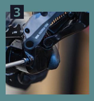
Find the black mounting screw at the bottom of the derailleur body. Use a T10 Torx screwdriver to remove the black T10 screw. Note that only half of the screw is threaded. Once the screw is about 1 cm out and the threads are no longer engaged, slide the screw the rest of the way out by hand. Keep the cage secure in the derailleur body with your thumb.
