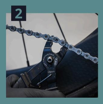
After installing the OSPW system, you will need to use a new, longer chain. Remove the old chain using a proper chain tool.
