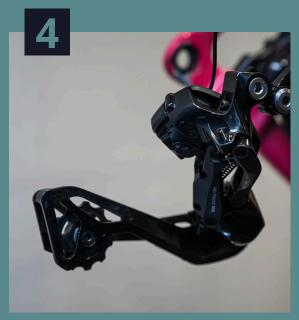
Shift the derailleur up so that the cage can rotate without hitting the derailleur body. For Ultegra 8150 or 105 7150, use a Phillips screwdriver to remove the rotation stop screw, then gently allow the cage to unwind. For Dura-Ace 9250, pull the cage away from the derailleur body by hand until the stop tower is free, then carefully let the pulley cage spring unwind to release the spring tension. At this point, your derailleur cage will appear upside down.
