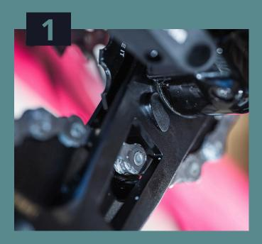
Position the chain on the smallest cog of the cassette and the small front chainring. To determine the correct chain length, bring the two ends of the chain together as you would when shortening a chain. The lower part of the cage should begin to move downward, away from the cassette. The stop pin of the cage should not touch the derailleur body.
