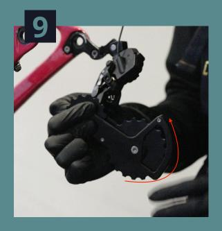
Hold the OSPW cage against the derailleur body and rotate it counterclockwise (first upward, then toward the back of the bike, and finally downward) until you feel the ramped stop tower click past the stop point on the derailleur.
