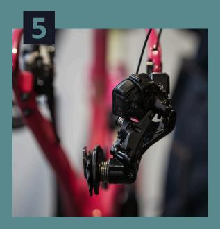
Slide out the original pulley cage and spring assembly, taking care not to drop the pulley spring or plastic spacer.
