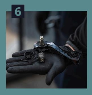
Remove the spring and plastic spacer from the Shimano cage. The spring's end is hooked to secure it in the pulley cage. Set these aside, as you will reuse them for the installation of the OSPW system.
