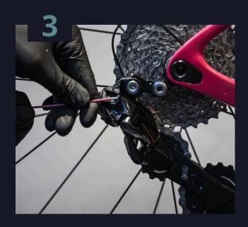
Set the b-limit gap between 4-7mm at the largest cog and upper pulley.
