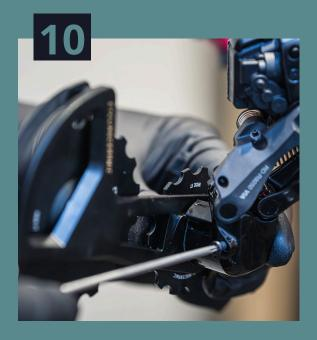
Secure the cage by reinstalling the original black T10 screw (removed in step 3). Tighten it to a torque of 1Nm. Your new OSPW system is now installed.
