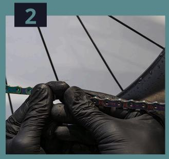
When tension is applied to the chain and the OSPW system appears the chain should be shortened by one link (compared to Step 1). Afterward, reconnect the chain with the appropriate number of links to achieve proper tension in this gear combination (always with the smallest cog on the cassette).
