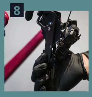
Choose the second spring tension hole from 'L' (second lowest tension) and fully insert the hooked end of the spring. You may need to press it firmly. The plastic spacer will rest loosely on the spring until it is aligned at the back of the derailleur body.
