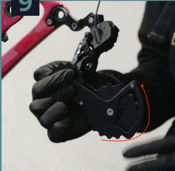
Hold the OSPW cage against the derailleur body and rotate it counterclockwise (first upward, then toward the back of the bike, and finally downward) until you feel the ramped stop tower click past the stop point on the derailleur.
