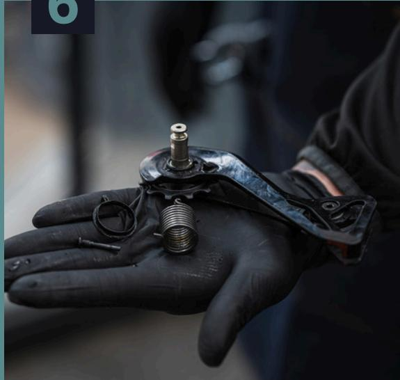
**Remove the spring and plastic spacer from the Shimano cage. The spring's end is hooked to secure it in the pulley cage. Set these aside, as you will reuse them for the installation of the OSPW system.**
