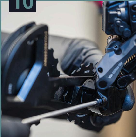
Secure the cage by reinstalling the original black T10 screw (removed in step 3). Tighten it to a torque of 1Nm. Your new OSPW system is now installed.
