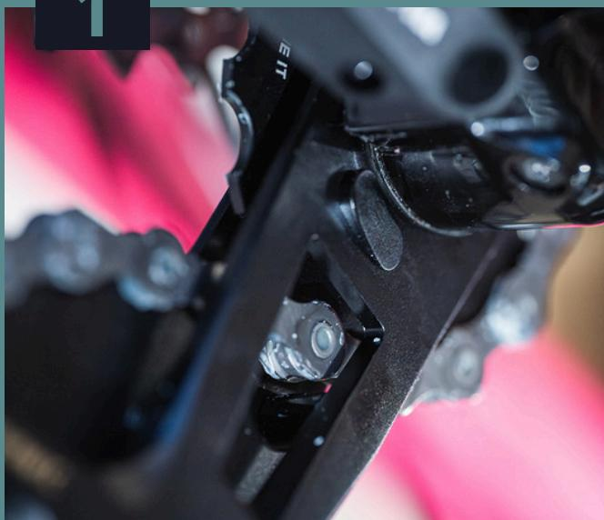
Position the chain on the smallest cog of the cassette and the small front chainring. To determine the correct chain length, bring the two ends of the chain together as you would when shortening a chain. The lower part of the cage should begin to move downward, away from the cassette. The stop pin of the cage should not touch the derailleur body.
