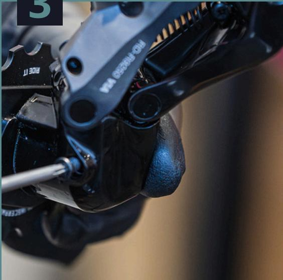
**Find the black mounting screw at the bottom of the derailleur body. Use a T10 Torx screwdriver to remove the black T10 screw. Note that only half of the screw is threaded. Once the screw is about 1 cm out and the threads are no longer engaged, slide the screw the rest of the way out by hand. Keep the cage secure in the derailleur body with your thumb.**
