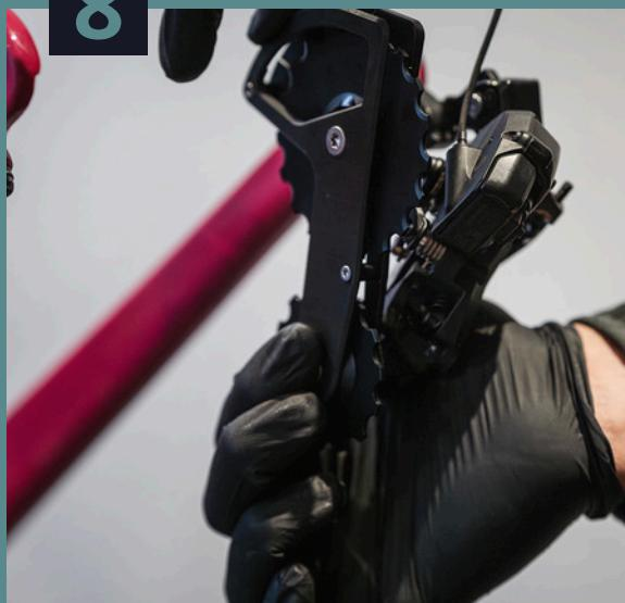
**Choose the second spring tension hole from 'L' (second lowest tension) and fully insert the hooked end of the spring. You may need to press it firmly. The plastic spacer will rest loosely on the spring until it is aligned at the back of the derailleur body.**
