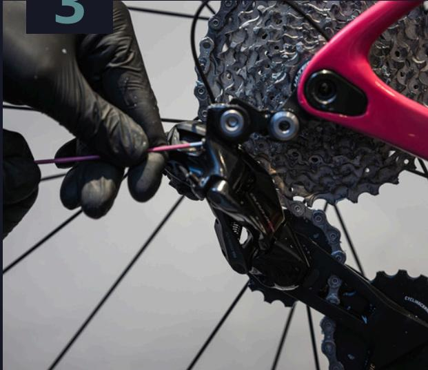
**Set the b-limit gap between 4-7mm at the largest cog and upper pulley.**
