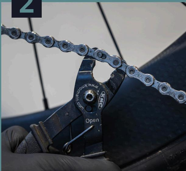
After installing the OSPW system, you will need to use a new, longer chain. Remove the old chain using a proper chain tool.
