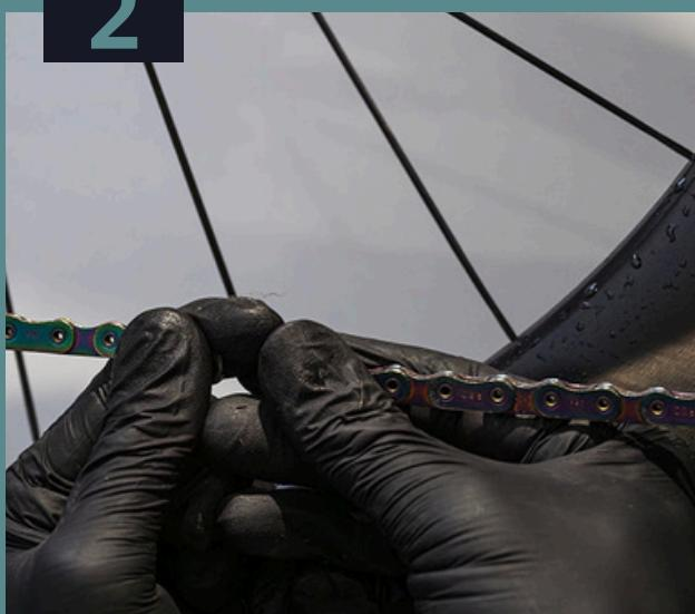
When tension is applied to the chain and the OSPW system appears the chain should be shortened by one link (compared to Step 1). Afterward, reconnect the chain with the appropriate number of links to achieve proper tension in this gear combination (always with the smallest cog on the cassette).
