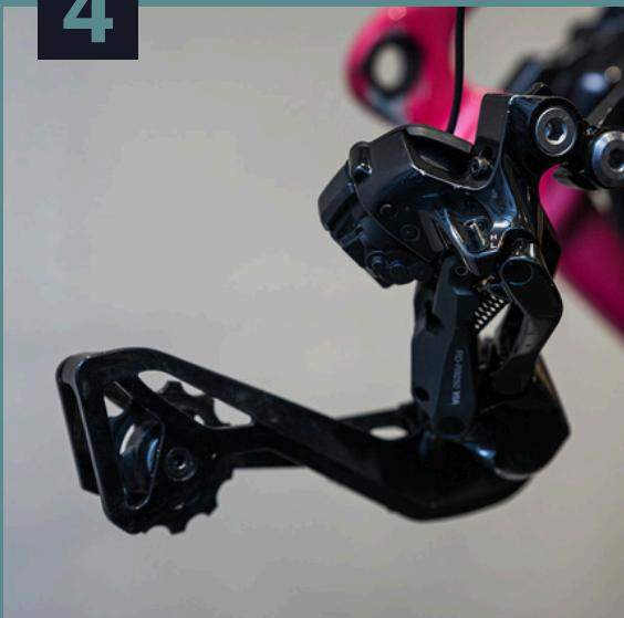
**Shift the derailleur up so that the cage can rotate without hitting the derailleur body. For Ultegra 8150 or 105 7150, use a Phillips screwdriver to remove the rotation stop screw, then gently allow the cage to unwind. For Dura-Ace 9250, pull the cage away from the derailleur body by hand until the stop tower is free, then carefully let the pulley cage spring unwind to release the spring tension. At this point, your derailleur cage will appear upside down.**
