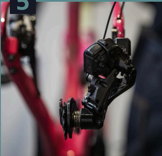
**Slide out the original pulley cage and spring assembly, taking care not to drop the pulley spring or plastic spacer.**
