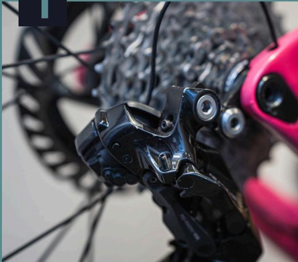
Start by placing your bike on a stand and removing the rear wheel.
